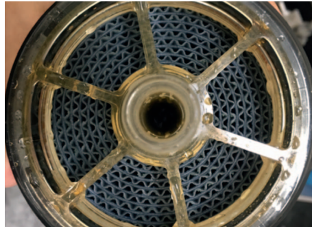
Figure 4: Open Channel Feed Spacer Design of Spiral Wound Monolith Element
