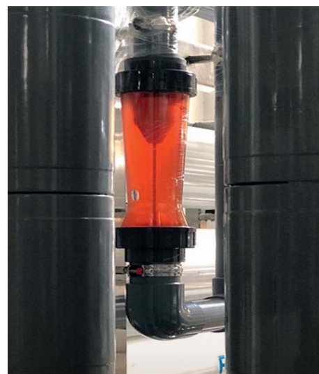
Inlet view of fermentation broth during batch processing, showing the feed stream prior to ultrafiltration.
